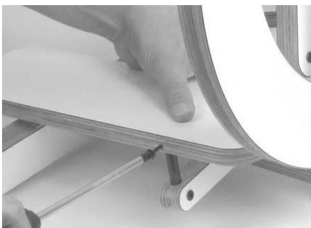
**EN** Insert both flexible pieces of the rocker arm into the holes of the treadles and be sure to press them to the bottom of the holes. Secure them using the 2 screws, left from hardware bag 2 .
