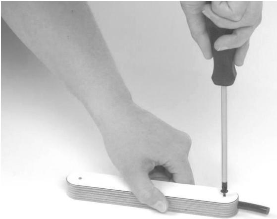
**EN** Open section 1 of hardware bag 1. Insert the flexible piece (the one without a hole) completely into the hole in the footman and screw in place with one of the screws  $3 \times 16$  mm.
