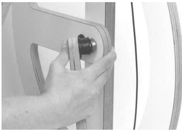
**EN** Place the drive band behind the footman and push the cup onto the eccentric bearing. It's easier if you hold the footman at an angle while you push it on. Secure the cup by pushing the ring to the edge.
