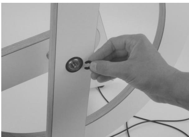
**EN** Mount on the main wheel to the front of the back post: Insert the axle through the ball bearings. Now push the wheel and post towards each other, so the spring is pressed together and the end of the axle protrude far enough to make it easy to push one of the retaining rings into the groove of the axle. This retainer has a small protruding edge for your nail to pull it out again; naturally this edge should face outside.
