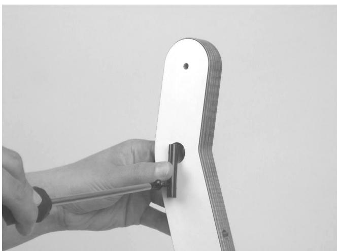
**EN** Open section 3 of hardware bag 1. Attach the flexible piece with screw 4 x 21 mm on the backside of the front post. The flexible piece should cover the middle of the hole. Tighten the screw firmly.
