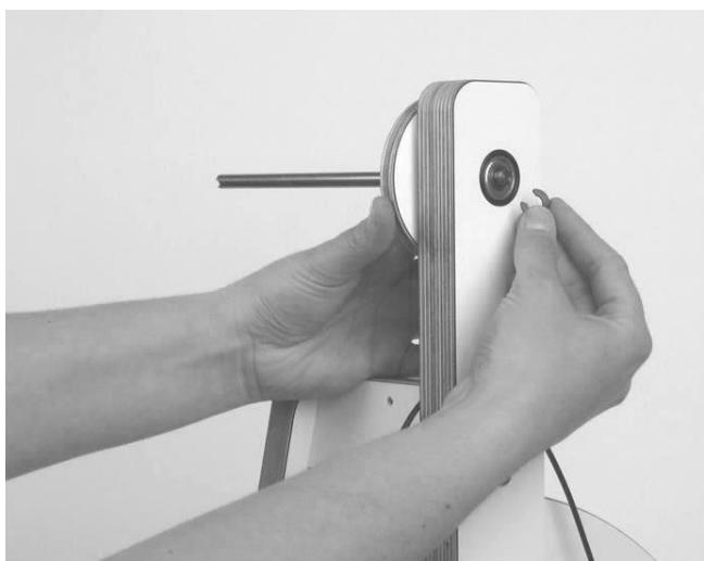
**EN** Insert the axle of the pulley through the bearings at the top of the back post and lock this assembly with the retaining ring, like you did for the wheel. There is a spare retaining ring left over in the hardware bag.
