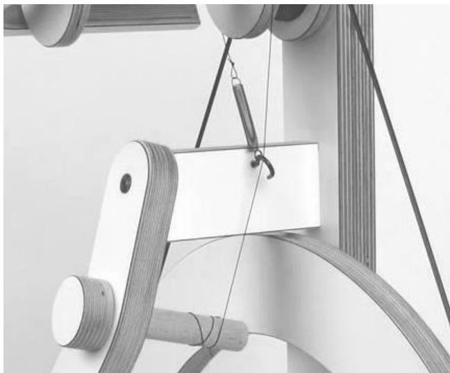
**EN** The spring should be on the left side (like in the left picture) when the wheel is turning clockwise when spinning and on the right when plying.
