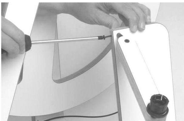
**EN** Place the flexible end of the footman in the hole of the right treadle, so the end is level with the bottom of the treadle and the cup on the footman is facing away from the treadle. Fasten the connection with the little screw, left from the first section of hardware bag 1.
