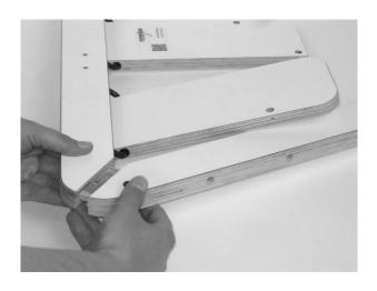
Disconnect the upright and the base piece of the front post by unscrewing the socket head screw.
