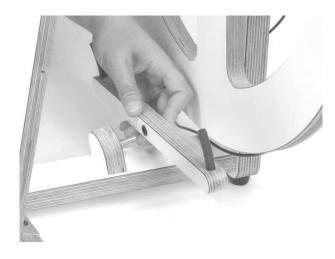
Remove the rocker bar from the axle of the hinge block.
