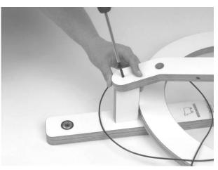
Remove the front post of the spinning wheel (together with the treadles) by unscrewing three screws; two at the bottom, one at the top.
