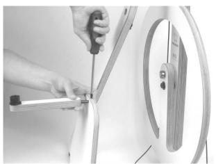
Place the flexible end of the footman in the hole of the treadle, so the end is level with the bottom of the treadle. Screw the footman to the treadle.
