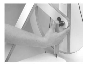
Place the drive band behind the footman and push the cup onto the eccentric bearing. It's easy if you hold the footman in an angle while you push it on. Secure the cup by pushing the ring to the edge.
