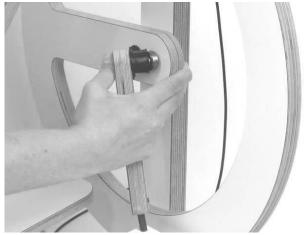
Detach the footman from the wheel by first pulling the ring from the eccentric cup back and then removing the eccentric cup from the bearing. This is easier if you force the footman at an angle while you remove the cup.
