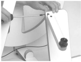
Detach the flexible end of the footman from the treadle.
