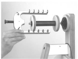
Re-attach the bobbin and the flyer onto the axle. The bobbin end with the groove should face the pulley.
