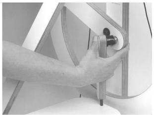
Detach the footman from the wheel by first pulling the ring from the eccentric cup back and then removing the eccentric cup from the bearing. This is easier if you force the footman at an angle while you remove the cup.
