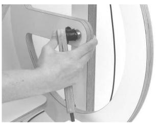
Place the drive band behind the footman and push the cup onto the eccentric bearing. It's easy if you hold the footman in an angle while you push it on. Secure the cup by pushing the ring to the edge.
