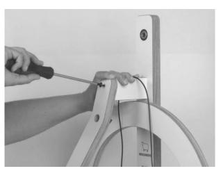
Add the drive band to the assembly and screw the front post to the upper rail and base rail.
