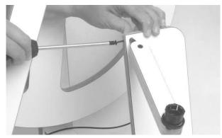
Insert the flexible piece of the footman into the hole of the right treadle, so the end is level with the bottom of the treadle and the cup on the footman is facing away from the treadle.
